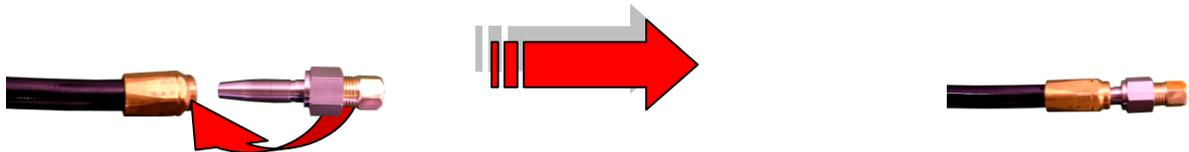
4. Unscrew the nut of the tapered adaptor. The connector is now ready for the hose from pump to membrane. We recommend using an insulating pipe to protect it against vibrations.
