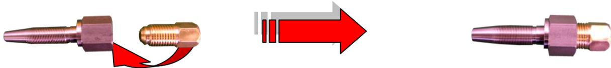
3. Lightly grease the tip of the stainless steel cone and screw it straight into the brass union. Stop where the steel threading disappears into the brass end-piece (a gap of approximately 7mm between the nut and the brass union)
