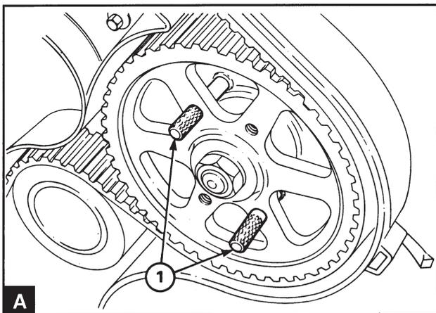
Install the two screws (M6 x 50) (A1) through the smooth holes in the fuel injection pump pulley and in the pump bracket.
