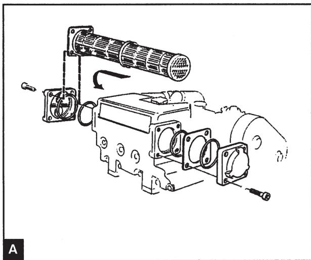
Remove the cover and press the insert out of the heat exchanger.
