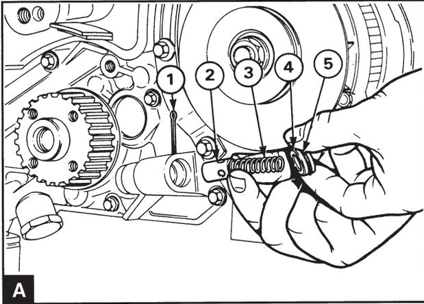
Bend the shafts of the split pin together (A1). Press the end plug (A4) and remove the split pin from the pump housing.
