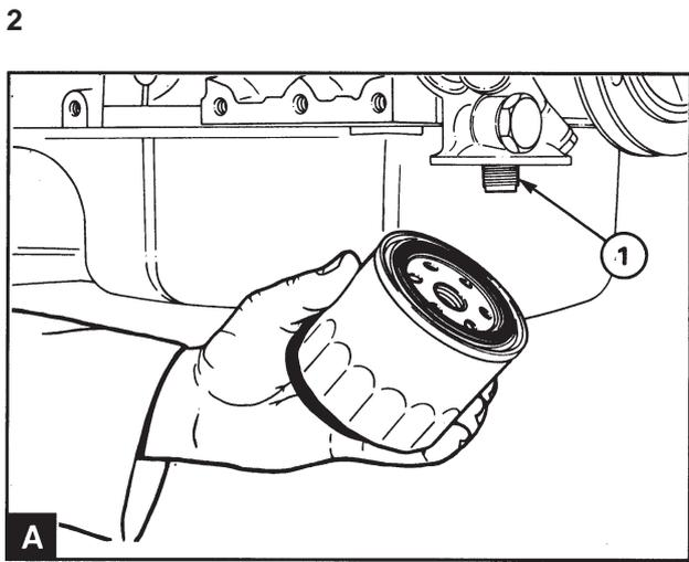
Remove the filter holder with a strap wrench or a similar tool. Ensure that the adapter (A1) remains in the filter head and discard the holder.
