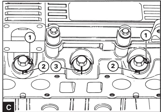
If the original screws have been reinstalled, mark the top of each screw with a punch mark to indicate that the screws have been tightened operationally. A maximum of four punch marks is permitted.
