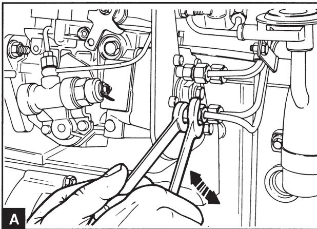
Remove all the necessary pipes from the pump. Use a wrench as a counterhold at the pump outlets side (A) to prevent the joint moving when the nuts for the delivery lines are slackened off.
