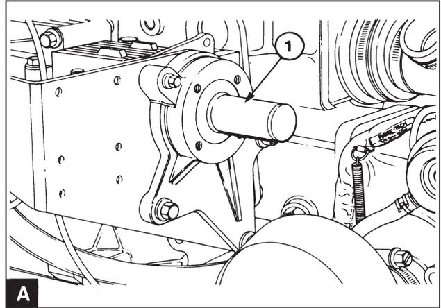
Position alignment tool 885038 (A1) with the narrow diameter in the camshaft and the wider diameter in the adapter plate. Tighten the mounting screws evenly in stages and remove the alignment tool.
