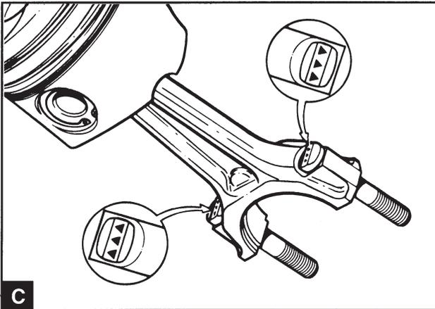
Check the condition of the connecting rod screws. If the thread is sealed or if there are signs of stretching, the screw must be removed from the connecting rod and replaced. The new screw must be installed with the locating arrows (or recognition marks) on the screw head turned to the outside of the connecting rod big end (C). Ensure that the screw head has good contact with the connecting rod.
