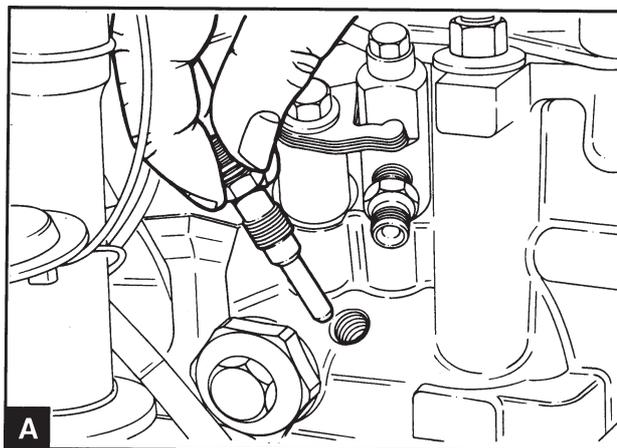
Disconnect and remove the plugs (A).
