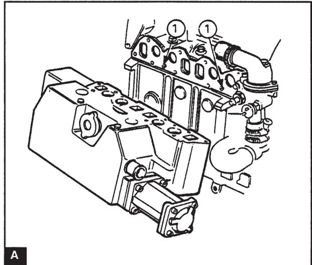
Unscrew the screws which secure the unit to the cylinder head evenly in stages in reverse order to the order shown in the illustration (B). Remove the unit (A).
