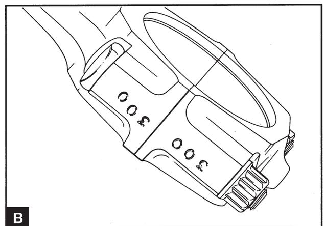
Clean the bearing shells and lubricate the bearing surfaces and big end journals. Install the upper bearing shell for the connecting rod with the locking lug well inserted in the cut out (A1). Install the connecting rod to the big end journal. Ensure that the marking on the connecting rod (B) lies in the same direction as the other connecting rods.
