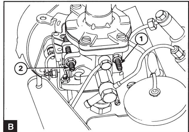
Run the engine to operating temperature and check the idling speed. If required adjustment can be carried out using the inner adjustment screw (B1). Slacken off the locknut and turn the screw clockwise to increase and counter-clockwise to decrease the engine speed (RPM). Tighten the locknut when the engine speed (RPM) is correct.
