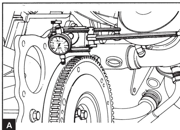
Check the radial run-out of the flywheel using a dial indicator (A). The run-out must be less than 0.30 mm as a total reading on the indicator.
