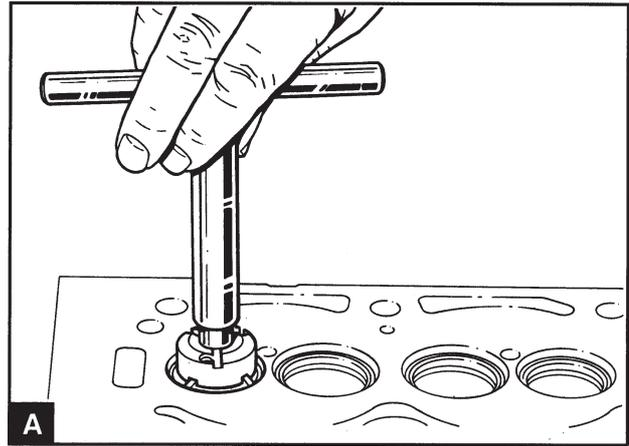
Install the mill on the locating pin with 46° side against the valve seat and install the handle (A). Do not let the mill head fall down towards the seat, this can damage the blade.
