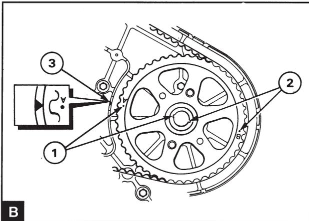
Install the pulley in position on the shaft with the correct keygroove in contact with the key. There are two keygrooves and two marked teeth, "A" and "B", on the pulley. On engines types MD22 and MD22L use the keygroove lying on the same side as the tooth marked "A". On engines types TMD22 and TAM22 use the keygroove lying on the same side as the tooth marked "B". Ensure that the marking on the pulley is turned to the front end of the engine.
