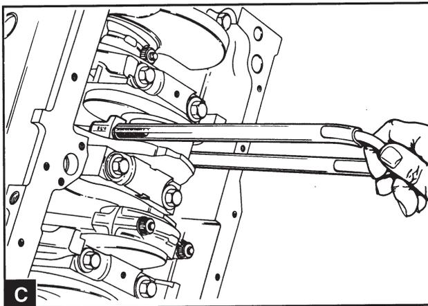
Install rubber or plastic protective tubes on the connecting rod screws (B1). Slide the piston and the connecting rod upwards in the cylinder bore. A suitable tool for this job can be made from a (U) shaped pipe and two pieces of plastic hose (C).
