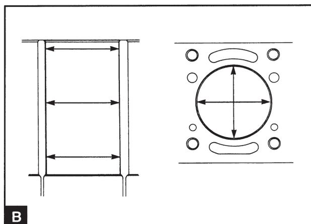
If the cylinder bores are damaged or worn more than 0.15 mm, measured in the diameter, the bore can be bored out and honed to 0.50 mm, diametrically oversize, and oversized pistons can be installed. For best results the cylinder bore should be honed with a total angle of 30° to 35° with a silicon carbide honing element which gives clean scoring. Coarse hone with a surface evenness of 1.5-2.0 mm (micrometer) and then fine hone to an mean
