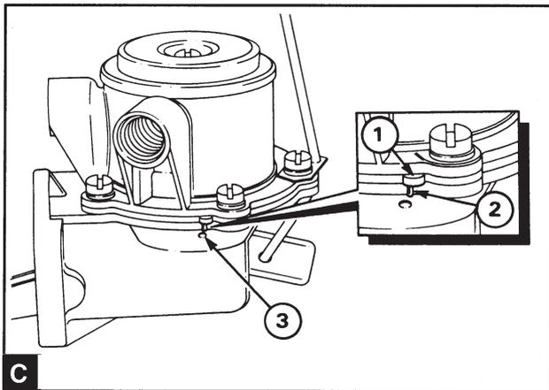
Press the rocker arm upwards in the diaphragm until the diaphragm lies at the level of the pump housing flange. Install the upper half of the pump housing in position with the marks on the flanges lined up. Keep pressure on the rocker arm and install the spring washers and screws. Remove the pressure from the rocker arm and tighten the screws evenly. After installation the edge of the membrane should lie along at the level of the edge of the pump housing.
