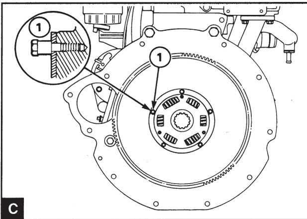
Install the elastic disc for the reverse gear (C). Apply Loctite 243 on the threads of the mounting screws for the disc. Ensure that the small guide section of each mounting screw goes into the flywheel (C1). Tighten the mounting screws evenly in stages to **9 Nm**. Do not start the engine until the locking fluid has hardened.
