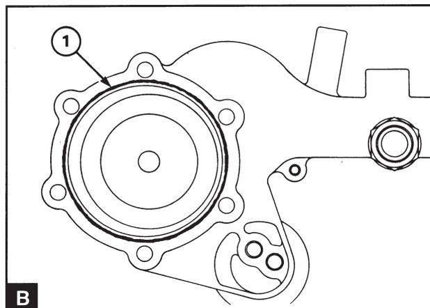
Apply a 1.0-1.5 mm continuous line of sealant on the pump mating surfaces, on the impeller side of the mounting holes (B1). If the old mounting screws are to be used, clean the threads of the screw which is to be installed at the "10 o'clock" position (A1) and apply sealant to the thread. Place the pump in position and tighten the mounting screws immediately after applying the sealant. Tighten the screws evenly in stages using the correct torque, see section 11B.
