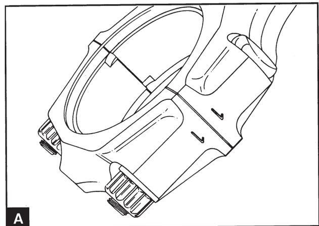
Check that all the connecting rods and the caps are marked with the correct cylinder number (A). If they are not marked, mark them from 1 to 4 with the number 1 at the timing belt cover end.
