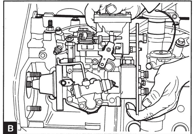
Remove the locknuts and remove the pump (B) – ensure that the key does not fall out of the drive shaft.
