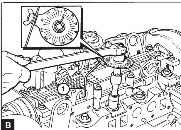
If no tool is available make a suitable marking on each screw flange (C1). Make other markings on the cylinder head (C2) with 90° clockwise offset in relation to the markings on the screws. Tighten each screw in the correct order until the markings on the screw match the markings on the cylinder head (C3). The screws do not need to be post tightened with the engine at operating temperature or after a certain period of operation.
