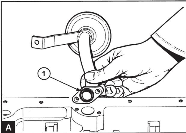
Remove the screws at the suction pipe flange and remove the suction pipe and screen. Remove the O-ring (A1). Clean the flange surface on the cylinder block and the suction pipe.
