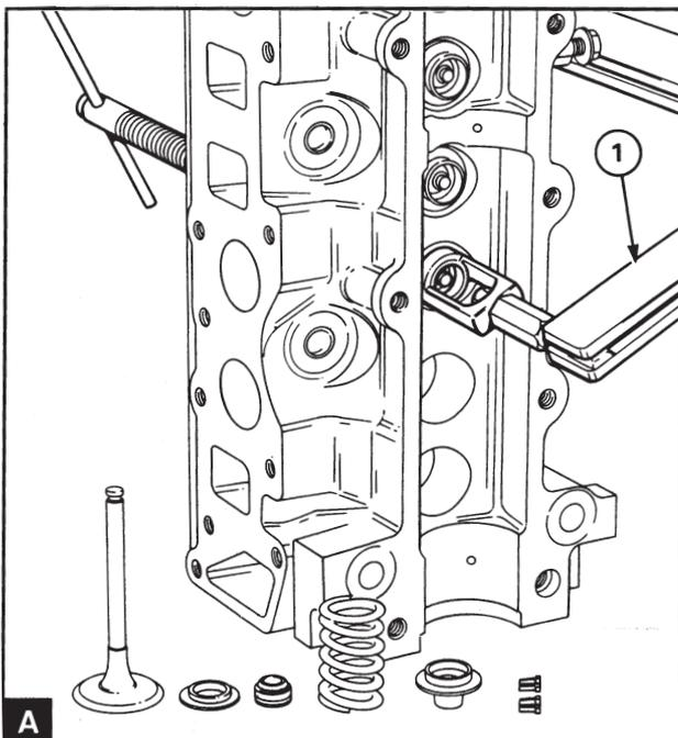
Press the valve springs together with the valve spring tensioners (A1). Ensure that the spring is pressed straight downwards so that the valve stem is not damaged. Remove the valve cotter (B1).
