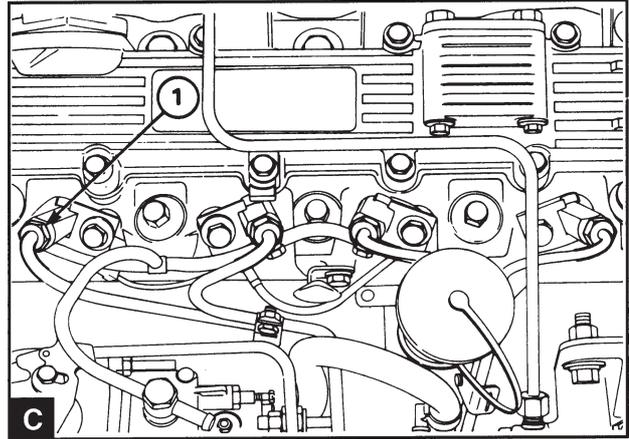
Slacken off the connector nuts for the delivery lines at the injectors (C). Depending on the type of injectors the connector nuts can be located above or beside the injectors.
