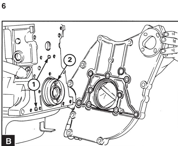
Check that the guide pins (B1) are correctly installed. Check that the outer diameter of the crankshaft flange is clean. Install the protective sleeve for the stuffing box (B2) in position on the crankshaft flange. Lightly lubricate the outer diameter of the crankshaft flange and the protective sleeve with fresh engine oil.
