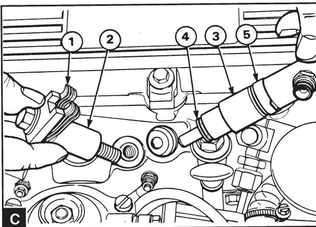
Slacken off the mounting screws for the injector holders. The spacer piece (C2) should either be 31.5mm or 7 mm long, depending on which type of injector is used. If a short spacer is used, lift the spring unit when the mounting screw is removed. This ensures that the mounting screw threads do not go in the hole in the lower spring. Remove the holder (C1) and the spacer washer. Remove the injector (C3) and the seat gasket (A4).
