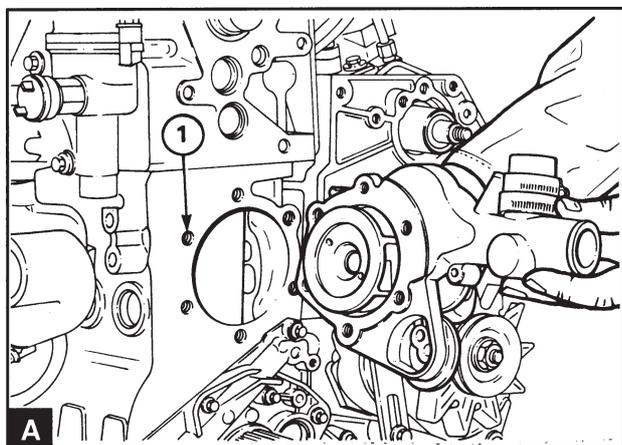
Remove the timing cover, operation 15A-08. Remove the pump mounting screws and remove the pump (A).
