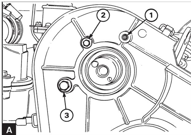
Remove the mounting screw which is installed through the camshaft cover into the timing cover (A1).
