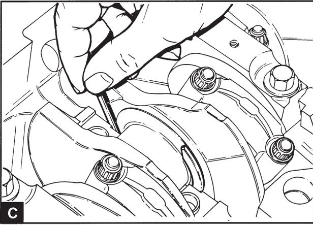
Remove the screws for the central main bearing and remove the bearing cap assembly with the three lower thrust washer halves (B). Press down one end of each and every one of the upper thrust washers with a suitable tool, made of soft material so that the relevant thrust washer slides out of its groove (C). If necessary move the crankshaft forwards or backwards to take the load off a thrust washer which is trapped.
