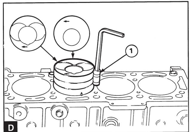
Ensure that the piston ring gaps are offset by 120° and press the rings together with a piston ring compressor (D1). Ensure that the protruberances pressed against one edge of the tool are bent downwards.
