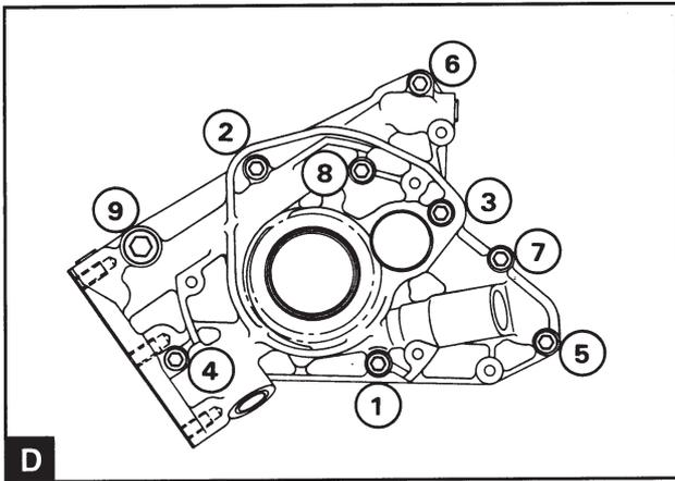
Install the pump mounting screws in position with a suitable sealing compound applied to the mounting screw which passes into the main bearing (D1). The sealing compound is already applied to new mounting screws. Tighten the screws in stages and evenly to the correct tightening torques, see Workshop Manual "Technical Data", in the correct order (D).
