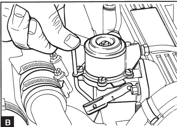
Pump the supply pump (B) with the lever until air free fuel comes out of the bleed screw. Tighten the bleed screw on the filter. If the supply pump drive cam is in position for maximum cam lift it is not possible to pump by hand. In this situation the crankshaft must be turned one revolution.
