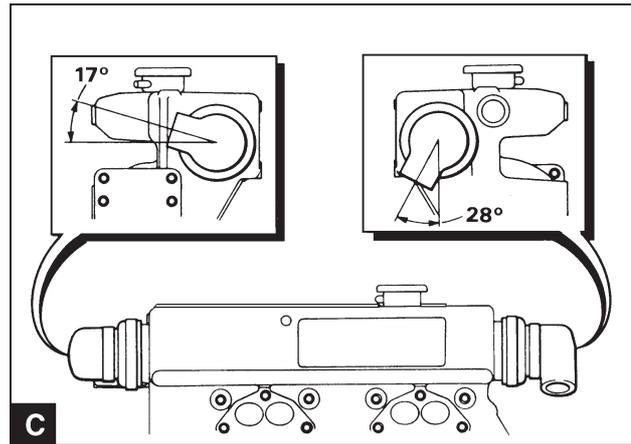
Install the second rubber end. Check that the pipe connectors of the rubber ends are in the correct position and tighten the clamps. Place the rubber ends in the positions shown in C if the assembly has been removed from the engine.
