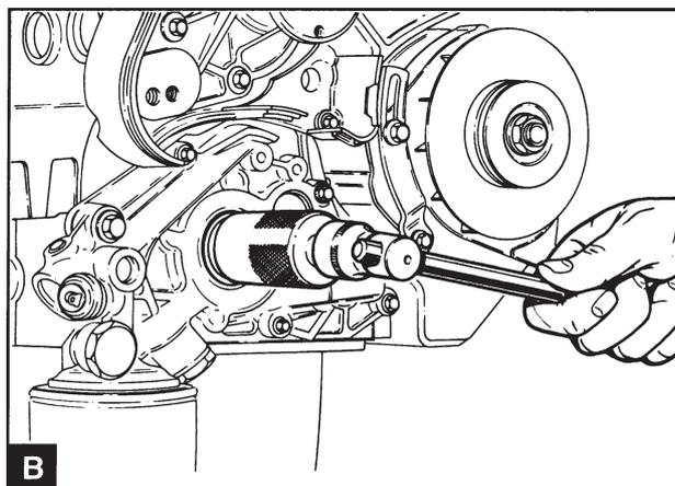
Install the adapter (A1) from the tool 885031 at the front end of the crankshaft. Slacken off the center screw so that it does not reach the adapter and insert the main tool in the sealing ring. Turn the tool clockwise to ensure that it is secure in the sealing ring and tighten the center screw against the adapter to remove the sealing ring (B). Remove the adapter.
