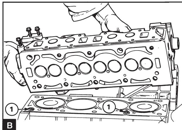
Unscrew the screws for the cylinder head evenly in reverse order compared to the illustration 12A.09/A. Remove the screws and dismantle the cylinder head (B), ensure that the camshaft does not come into contact with the timing cover. Place the cylinder head on even surface that will not damage the cylinder head surface.
