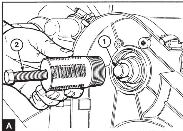
Install the plug from the tool 885026 (A1) in the front end of the camshaft. Unscrew the center screw (A2) sufficiently to ensure that it does not reach the plug and insert the main tool into the stuffing box. Turn the tool clockwise to ensure that it is secure in the stuffing box and tighten the center screw against the plug to remove the stuffing box.
