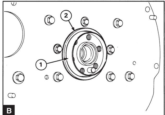
Clean and lubricate the protective socket 885030 (B1) and install it on the end of the crankshaft flange.
