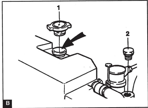
Remove the bleed plug from the outlet connection for the coolant (B2).
