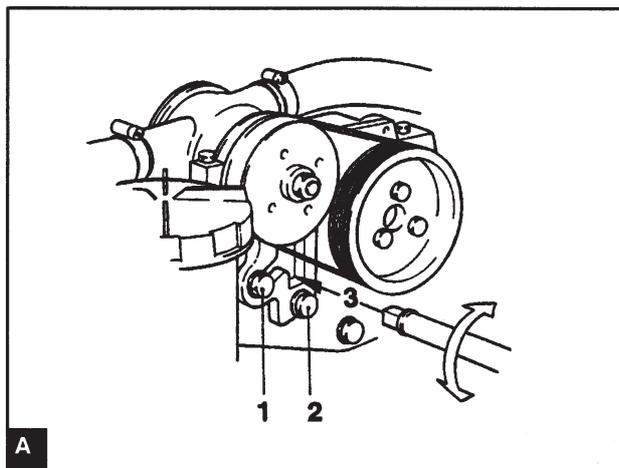
Detach the two mounting screws (A1) and (A2) and remove the belt. Remove the pump.
