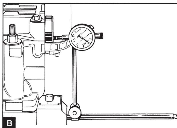
Check the camshaft axial clearance with a dial indicator (B). For tolerances see Workshop Manual "Technical data".
