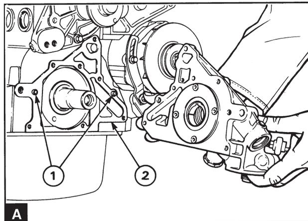
Check that the mating surfaces of the oil pump, cylinder block and main bearing cap are clean. Check that the two guide pins (A1) are in position and install a new gasket (A2).
