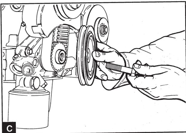
Slacken off the pulley center screw and remove the pulley (C). Use a large screwdriver or similar tool as a counterhold at the flywheel ring gear.
