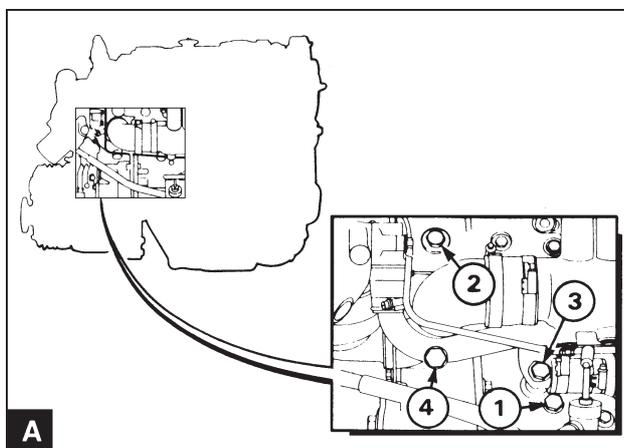
Drain the coolant by removing the plug (A1) on the starboard side of the engine block. Ensure that the drain hole is not blocked by contaminants.
