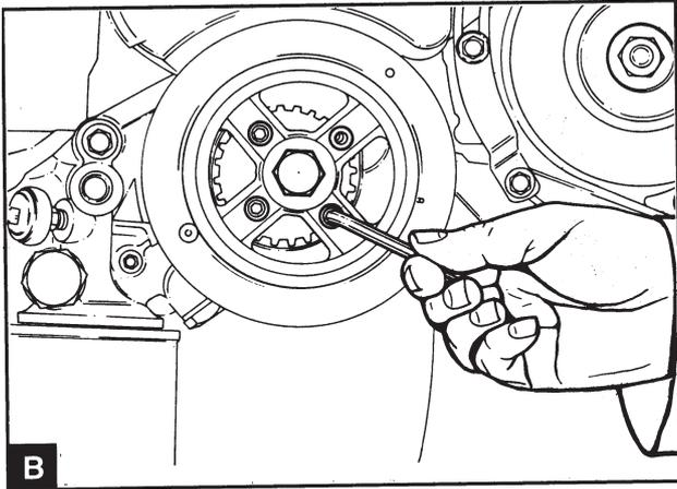
Unscrew and remove the four mounting screws (B) which secures the pulley to the belt pulley.
