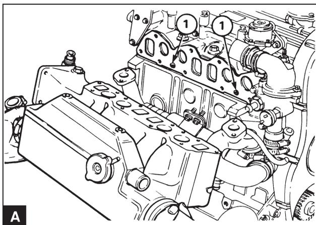
Unscrew the screws which secure the unit to the cylinder head evenly in stages in reverse order to the order shown in the illustration (B). Remove the unit (A).
