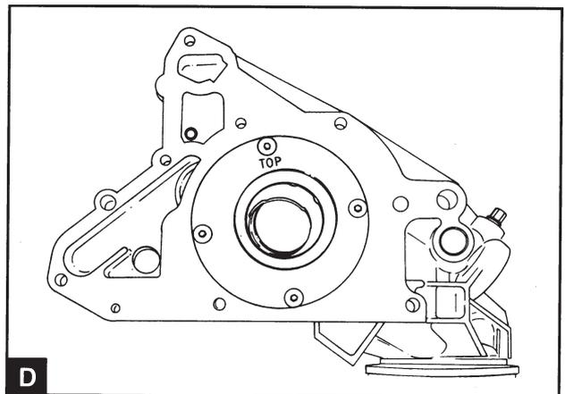
Lightly apply fresh engine oil to the rotors and insert them in the pump. The inner rotor has a lug in one end and this tap must be turned towards the sealing ring housing. Install the back plate with the word "TOP" turned from the pump housing straight edge (D). Install and tighten the screws for the back plate to **4 Nm**.
