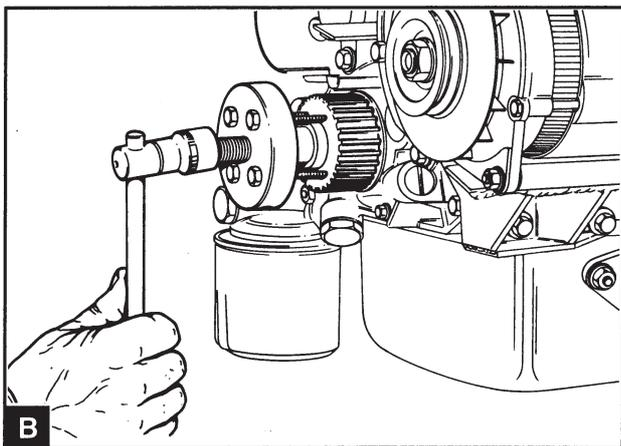
Insert the thin end spacer piece in the crankshaft (A1). Install the main tool 885027 (B) on the pulley using the mounting screws and tighten the center screws against the spacer piece to remove the pulley.
