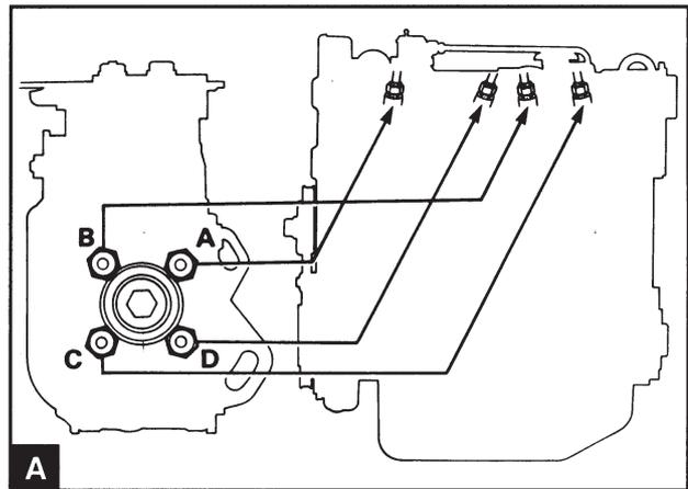
Install the delivery pipes to the pump. Use a wrench to prevent the output terminals on the fuel pump (FP) from moving when the delivery lines are installed. The connections to the pump are as displayed in illustration A. Do not tighten the connector to the injectors until the system has been bled.
