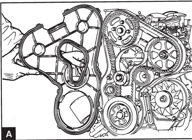
Remove the clips for the cover and remove the cap (A).
