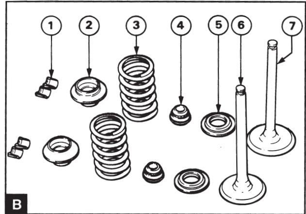
Take the load off the valve spring tensioner and remove the valve spring washer (B2), valve spring (B3), valve stem seal (B4) and the spring seat washer (B5). Remove the exhaust valve (B6) or the inlet valve (B7).
