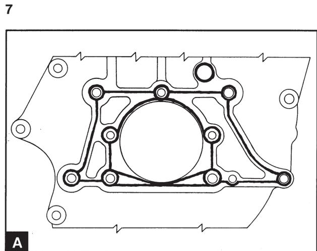
Apply a continuous 1.5 mm line of sealant on the front surface of the cover, as shown in illustration A. This operation is not necessary if a separate housing is installed for the stuffing box.
