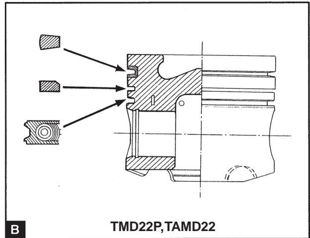
Install the "barrel face" ring with the molybdenum insert in the upper piston ring groove (TMD22P, TAMD22 Keystone ring). The word "TOP", the manufacturers mark or the internal milling must face the top of the piston. The new piston rings have a red identification mark. This must lie to the left of the ring gap when the ring is installed and the piston is raised.
