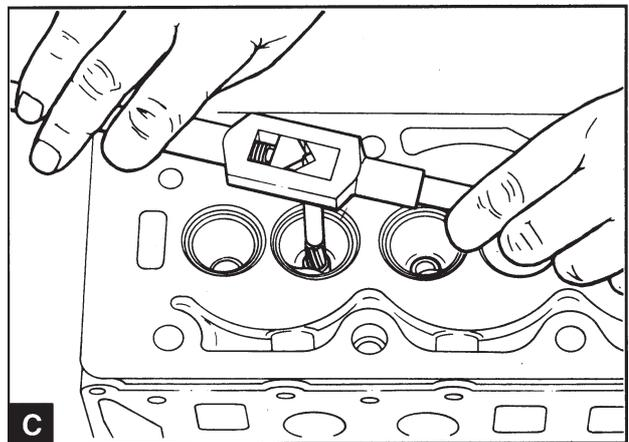
Ream the hole for the new guide using reamer 885022 (C).
