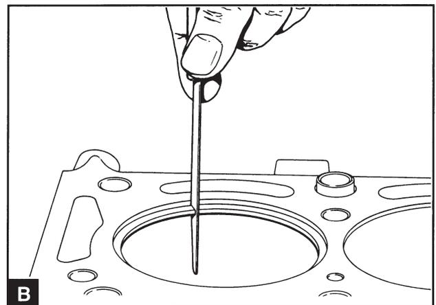
Check that all the soot has been removed from the upper section of the cylinder bore. Install the piston rings in the upper section of the cylinder bore and measure the ring gap with a feeler gauge (B). The expander ring must be installed on the oil scraper ring when the ring gap is measured. The ring gap for the new components is given in the Workshop manual "Technical data".
