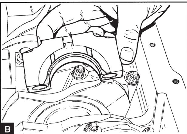
Install the lower thrust washer halves in the main bearings with the lugs in their respective cut outs. Check that the lubrication grooves in the thrust washers are turned away from the bearing cap (B).
