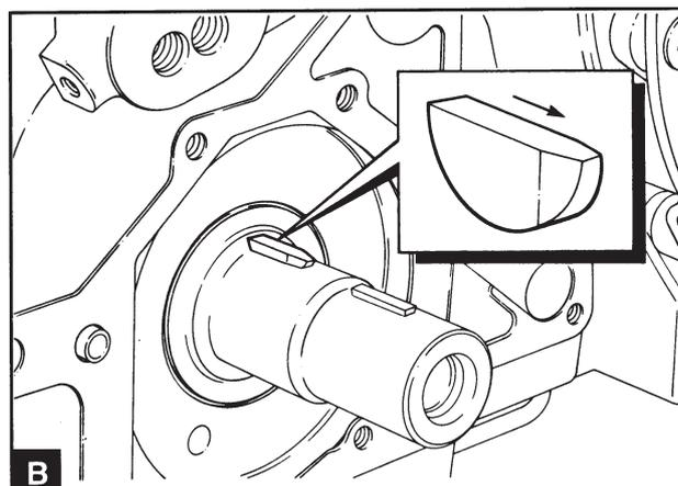
Ensure that the rear key is in position and that the bevelled end of the key is turned forwards (B). If the front key is still in position, remove it from the crankshaft.
