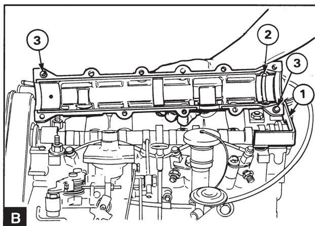
Remove the engine lifting brackets. If nothing is driven from the rear end of the camshaft, remove the rear cover and install the camshaft lock 885025 (B1). This ensures that the camshaft does not tilt when the camshaft cover is removed.
