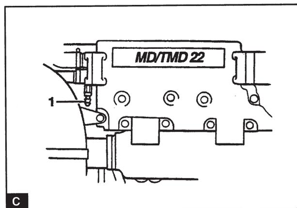
Drain the water from the heat exchanger (MD, TMD) through the cock (C1).
