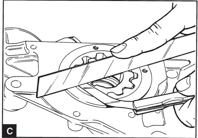
If the sealing ring needs changing, remove the rotors and press the sealing ring out of the housing. The pump is easier to install on the engine with the sealing ring uninstalled and the sealing ring can be installed on the installed pump, see operation 14A-02.
