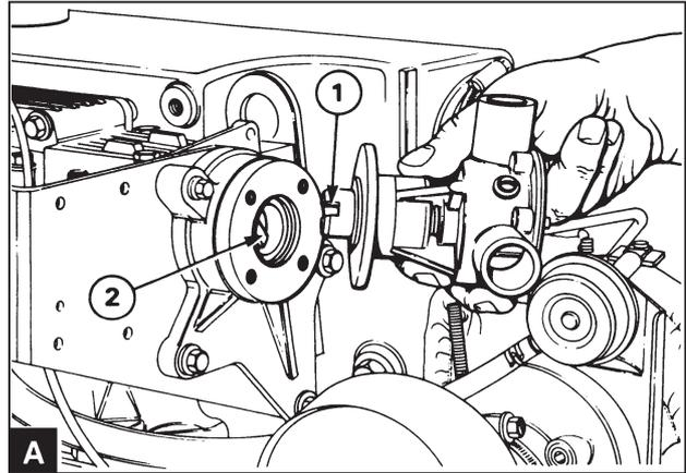
Align the cut out in the pump shaft (A1) with the flange driving pin (A2). Install the pump on the engine with a new gasket between the pump and the adapter plate. Install the mounting screws and tighten to **9 Nm**.
