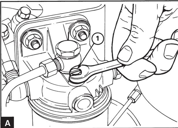
Slacken off the bleed screw (A1) located above the fuel filter, two or three turns.
