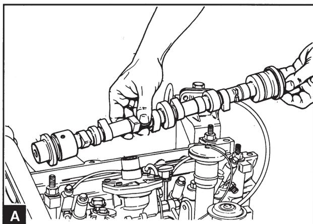
Remove the camshaft (A) and remove the camshaft sealing rings.
