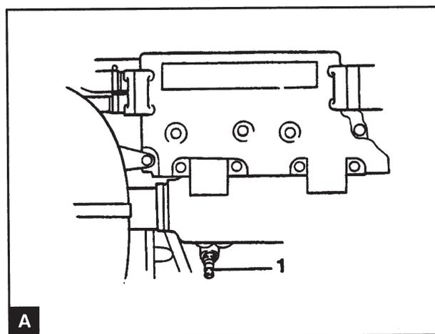
Drain the coolant using the cock (A1) on the starboard side of the engine block.
