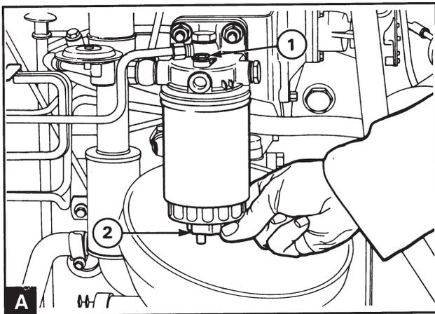
Carefully clean the outside of the fuel filter unit. Slacken off the bleed screw (A1) located above the filter, two or three turns. Slacken off the drain arrangement (A2) at the bottom of the holder and drain the fuel into a suitable container.
