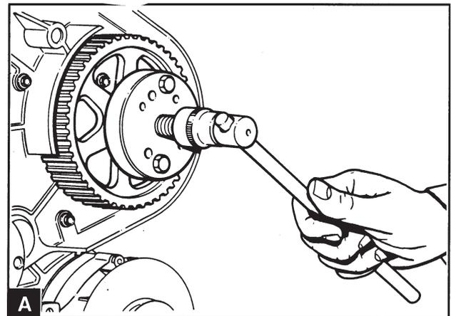
Remove the pulley with pulley puller 885027 and adapters 885029. Take care not to lose the key.
