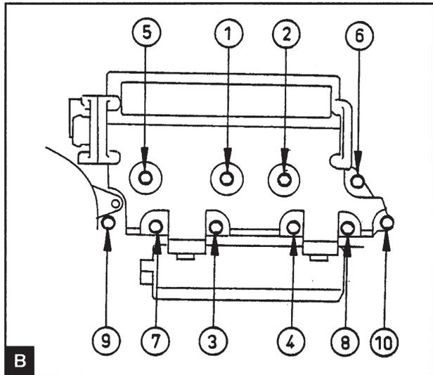
Place the unit in position on the cylinder head and install the mounting screws. Tighten the screws evenly in stages to **22 Nm** in the order illustrated in B.
