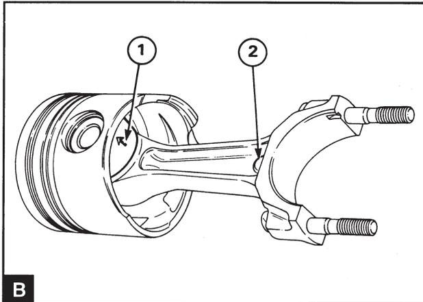
Place the connecting rod with piston upside down. The locating lug (B2) on the connecting rod must be on the same side as the arrow (B1) on the underside of the piston.
