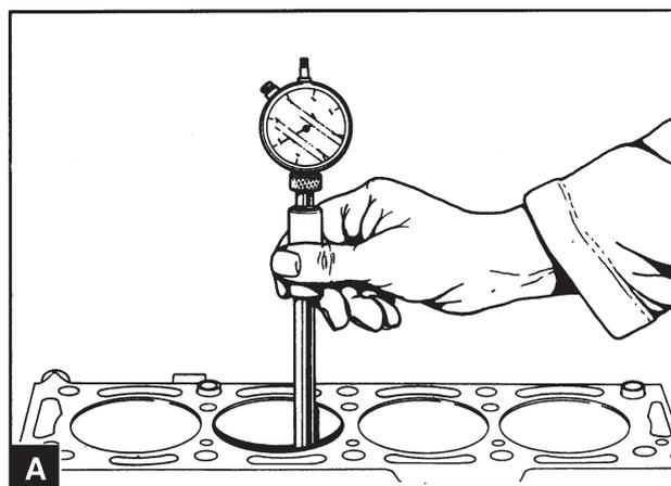
Check the cylinder bore for wear (A) and damage. The top, bottom and center of the cylinder bore should be inspected in both the vertical and lateral planes (B).
