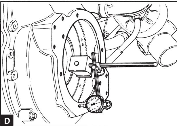
Install the flywheel and the drive adapter for the reverse gear, operation 21A-01. Check that the guide pins are correctly installed in the housing. Install the adapter housing for the reverse gear and tighten the mounting screws to **43 Nm**. Check the concentricity of the housing (C) and the axial run-out (D) in the same way as in points 5 and 7 above. Install the support plate for the manifold.
