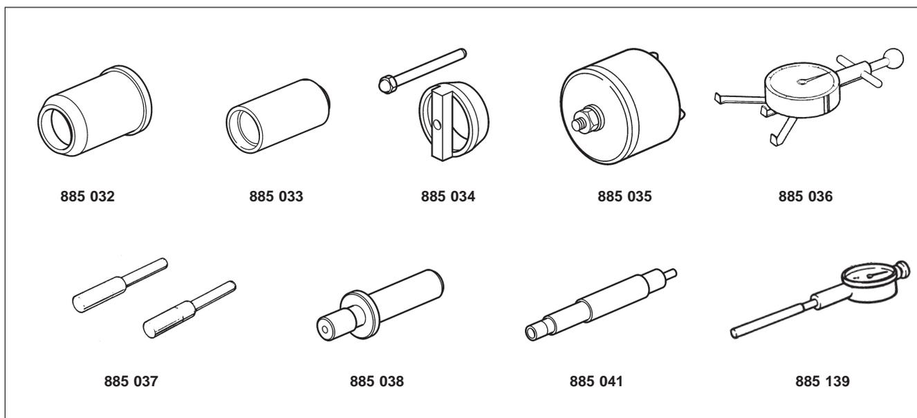
885032-3 Protective socket for front stuffing box, crankshaft.
