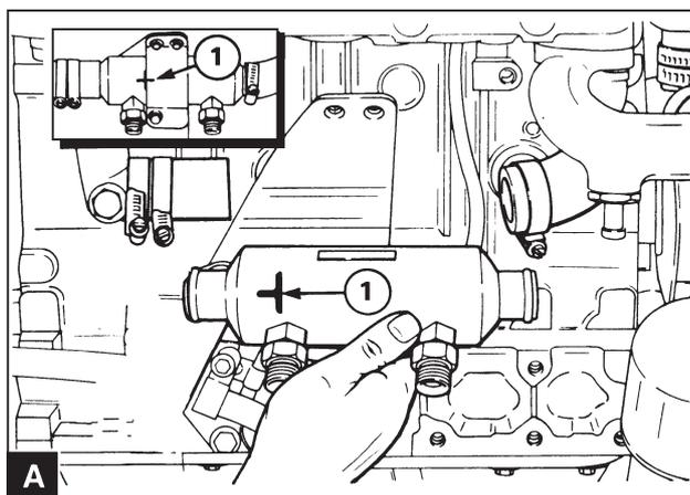
Make a mark with a felt-tip pen on the oil cooler housing and on the clamp (A1) in order to be able to reinstall the oil cooler in the same position.
