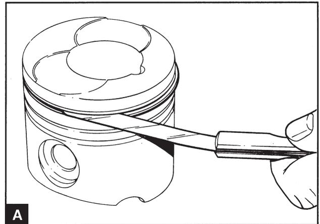
Install the new piston rings in the piston ring groove and check the ring groove wear using the feeler gauge (A). Compare the piston ring play in the groove to the values that apply to new components in the Workshop Manual "Technical Data". Replace the cylinder if necessary.
