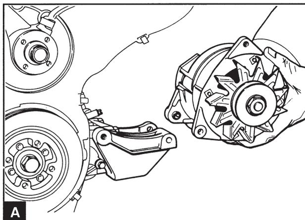
Remove the adjuster link from the generator and remove the pivot shaft. Note the position of the washer to ensure that it is correctly installed. Remove the generator (A).
