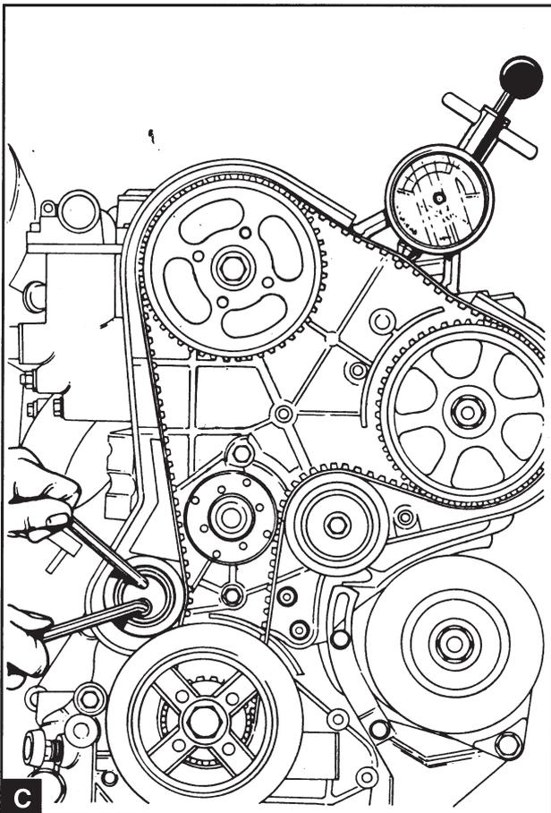
Unscrew the domed screws holding the belt tensioner roller. Adjust the belt tension using a hexagonal key in the hexagonal socket in the roller (C). The correct tension for a new belt is 425-465 N and for a used belt 340-370 N. When the tension is correct, tighten the domed screws to **45 Nm** and then recheck the belt tension.
