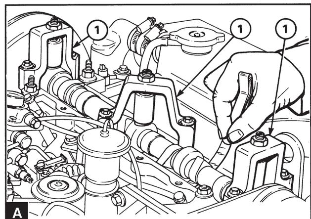
Install the camshaft mountings 885024 (A1) to hold the camshaft and mount the mountings with the relevant mounting screws for the cover. It is vital to move the rear camshaft stuffing box on the camshaft to secure sufficient clearance between the rear mounting and the stuffing box. Ensure that the sprung pads are correctly installed on the camshaft bearing journals and tighten the mounting screws for the mountings evenly.
