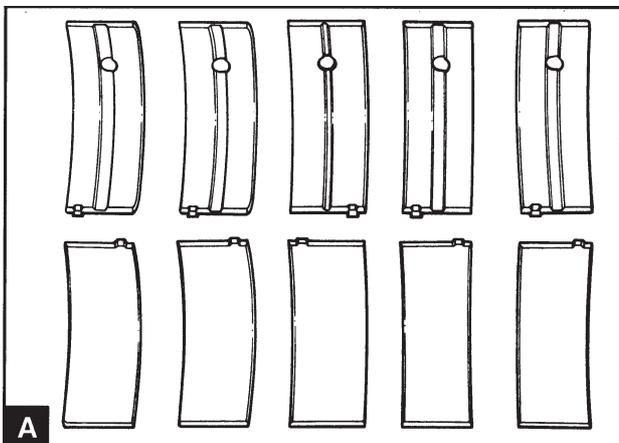
Clean the upper bearing shell and lubricate the bearing surface with fresh engine oil.
