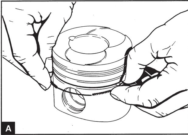
Insert the expander ring for the oil scraper ring in the lower piston ring groove with the catch through both end of the rings (A). Install the oil scraper ring over the spring (B). Ensure that the ring gap is located with a 180° offset to the catch.
