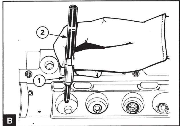
Install the guide B1 on the thin end of the tool 885021 (B2) with the bevel turned to the thin end of the tool (B). Insert the bevelled end of the guide into position in the cylinder head and press in the guide until the tool end comes into contact with the flat plate. Check that the guide protrudes 10 mm above the mating surface for the valve spring.
