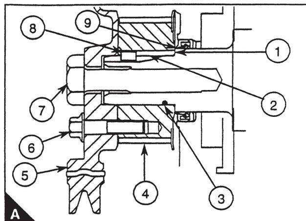
Apply a bead of Loctite 648 (A3) in a complete circle internally in the hole in the pulley (A4), 6.5 mm from the rear end panel.
