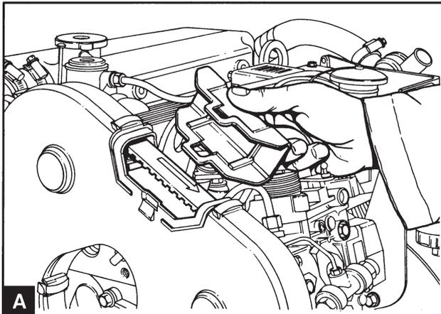
Remove the inspection hatch from the upper side of the timing cover (A).
