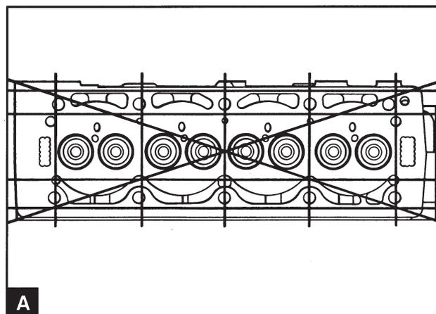
Use a straight edged ruler and a feeler gauge to check the latitudinal, longitudinal and diagonal flatness of the bottom surface of the cylinder head (A). If deformation is greater than 0.10 mm the bottom surface can be machined. Remove the minimum amount of material and check that the cylinder head height will not be less than 119.85 mm after the cylinder head has been treated.
