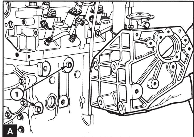
Install the fuel injection pump bracket. Check that the guide pins (A1) is correctly installed. Tighten the mounting screws to **43 Nm**.
