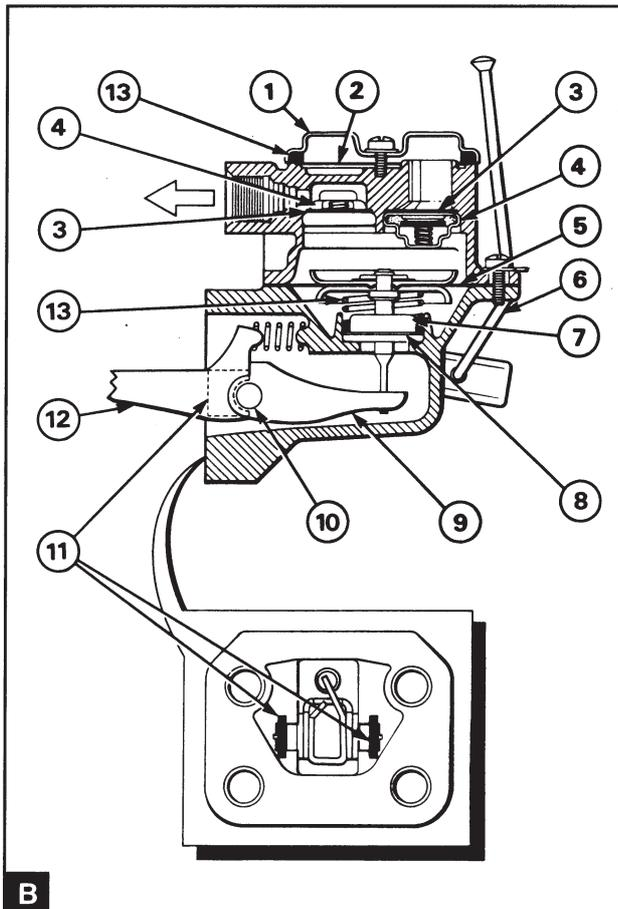
Remove the cap of the supply pump (B1) and the metal screen (B2). Remove the screws and separate the pump halves.
