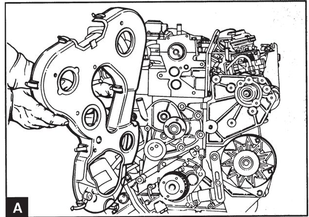
Unscrew the screws securing the timing cover to the cylinder head, the cylinder block, the fuel injection pump bracket and the oil pump. Remove the timing cover (A).
