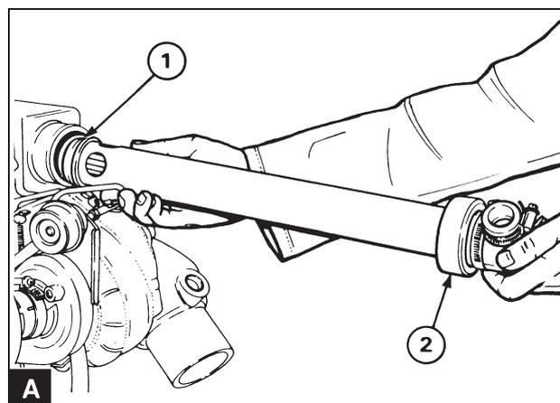
Press out the insert in whichever direction. Ensure that the sleeve (A1) also comes out of the heat exchanger.
