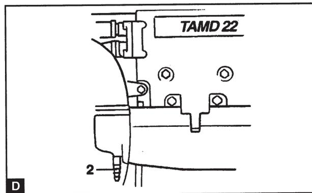
On the TAMD22 the water is drained through the cock (D2) on the charge air cooler (CAC).
