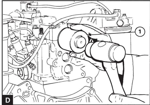
Ensure that the stuffing box and the camshaft are clean and undamaged. Lubricate the new stuffing box with fresh engine oil and insert it into position with the seal lip inwards. Use installation tool 885020 (D1) and a hammer with a soft face to drive the stuffing box into the correct position.
