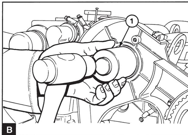
Ensure that the stuffing box and the camshaft are clean and undamaged. Lubricate the new stuffing box with fresh engine oil and insert it into position with the seal lip inwards. Use installation tool 885026 (B1) and a hammer with a soft face to drive the stuffing box into the correct position.
