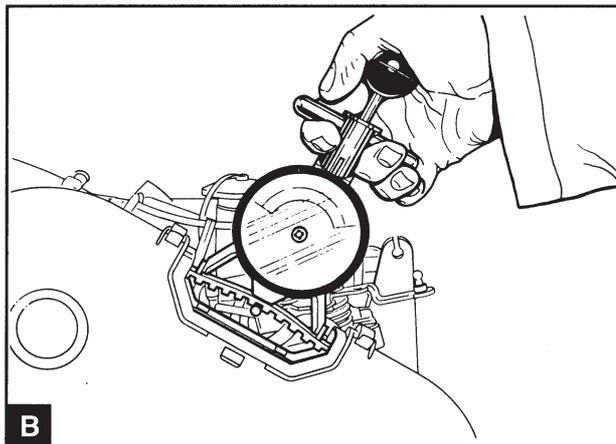
Press the ball end of the belt tension gauge and install the gauge over the belt. Ensure that the gauge foot is located under the belt and between two teeth (B). Slowly release the ball end and read off the gauge. Turn the crankshaft slightly in each direction until a stable read off is obtained. The correct value for a new belt is 425-465 N and for a used belt 340-370 N. If the tension of a used belt has fallen to 270 N or below, adjust the belt tension to 340-370 N, operation 15A-03.
