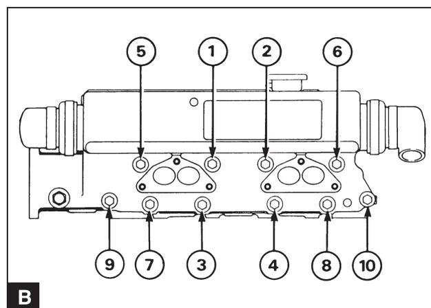
Place the unit in position on the cylinder head and install the mounting screws. Tighten the screws evenly in stages to **22 Nm** in the order illustrated (B).
