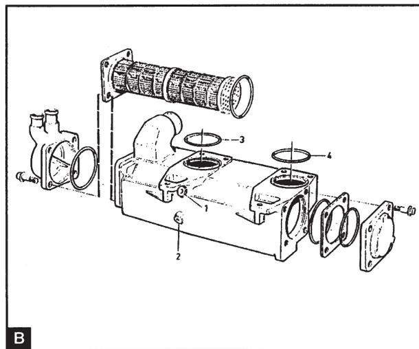
Remove the charge air cooler assembly from the heat exchanger. Remove the cover and the plugs (B1 and B2). Press the insert out of the heat exchanger.
