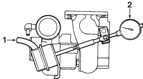
If the by-pass valve in the boost pressure control valve does not open at the correct pressure, this will affect the performance of the engine.
