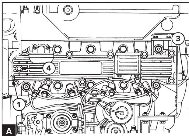
Remove the screws securing the camshaft cover front flange to the timing cover (A1).
