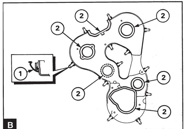
Check the timing cover for cracks and damage and replace it if required. Check that all the clips are correctly installed in the timing cover (B1).
