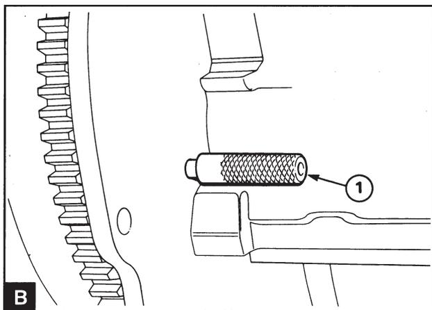
Install the adjustment drifts through the camshaft cover in the camshaft (A1) and through the flywheel cover in the flywheel (B1).
