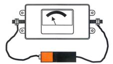
If the needle stays in the centre position and does not move then the unit should be removed from the safety earth as soon as possible and returned to Aquafax Ltd for testing.
