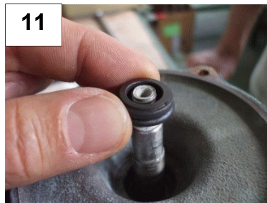
11 Deep the grafite part in water and then slide it on the shaft keeping the mirror finished surface towards you
