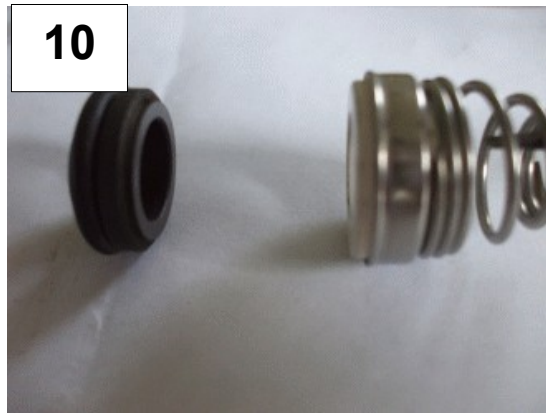
10 This is the new shaft seal – note the left grafite part with mirror finished surface and the right part which is rotating with the shaft
