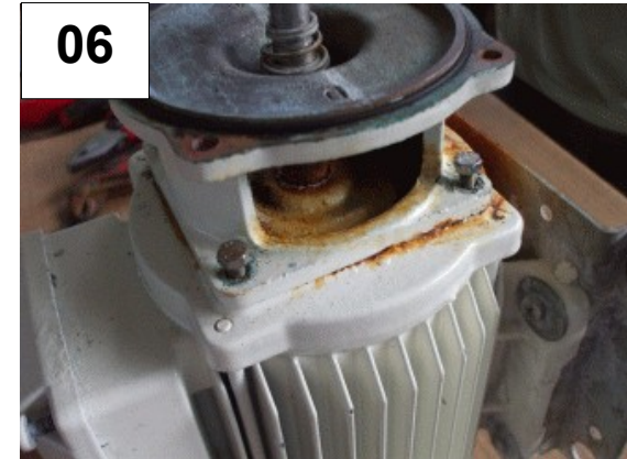
Back pump body removal
