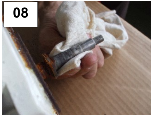
08 Shaft seal cleaning –
