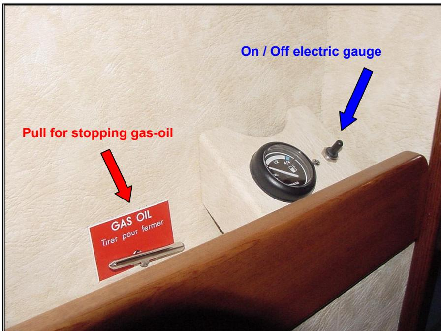
*Pict. 59 – Gas-oil electric gauge and lever for stopping gas-oil delivery from the passageway*
