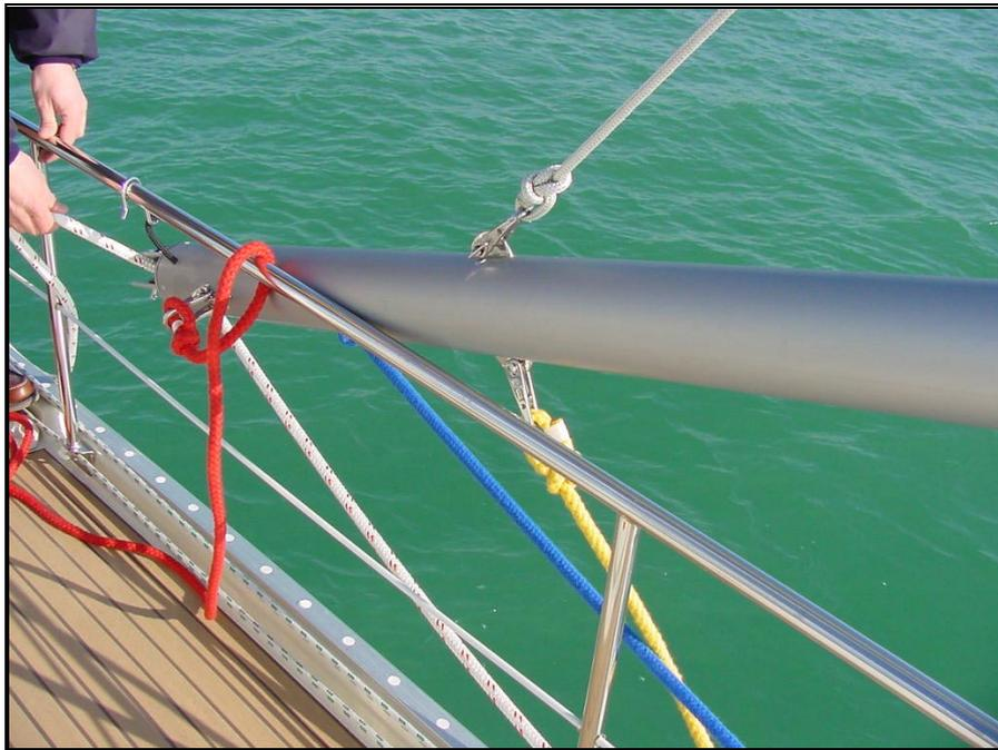
*Pict. 40 – Attachment of the lines on the pole and way of jib's sheet*
