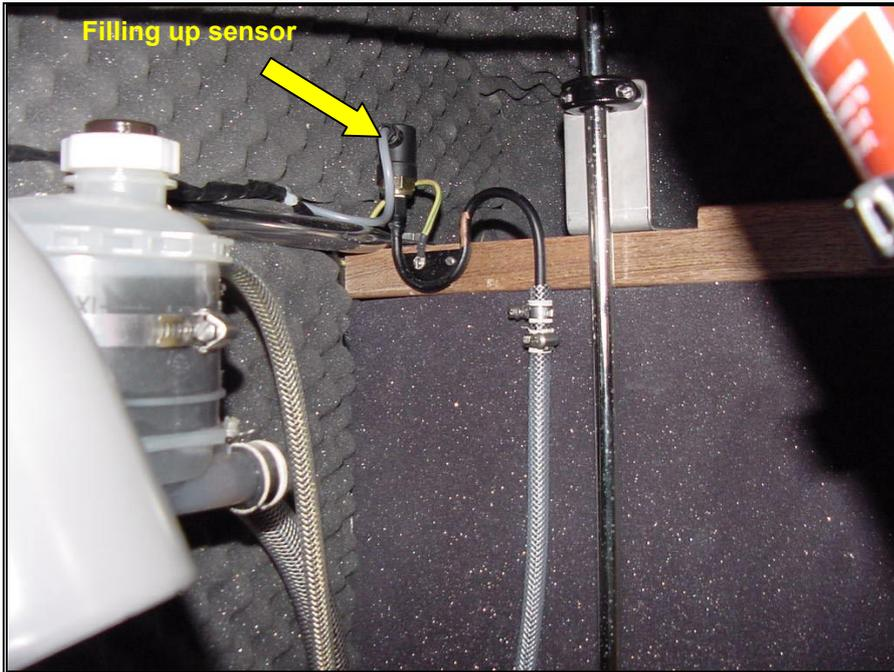
Pict. 65 – Blockage sensor of the seawater filter
