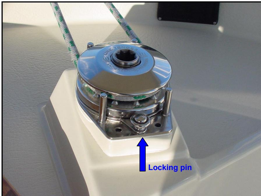
*Pict. 22 – Main sheet traveller control (locked on both ways)*
