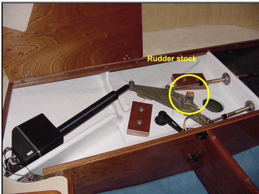
*Pict. 17 – Rudder stock and automatic pilot linear driving unit*
