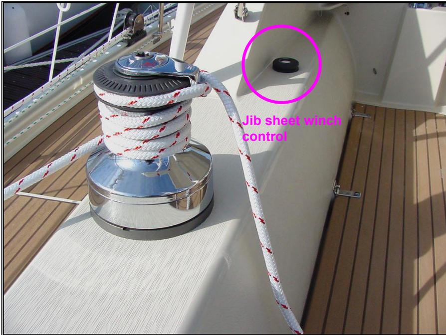
*Picture 11 – Jib sheet electric winch*
