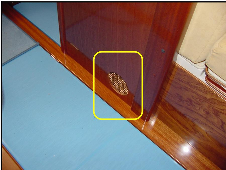
*Picture 76 – Clothes' washer / dryer intake*
