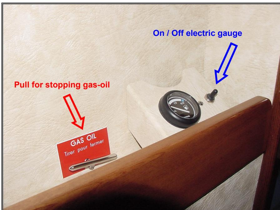
Picture 50 – Gas-oil electric gauge and lever for stopping gas-oil delivery from the passageway
