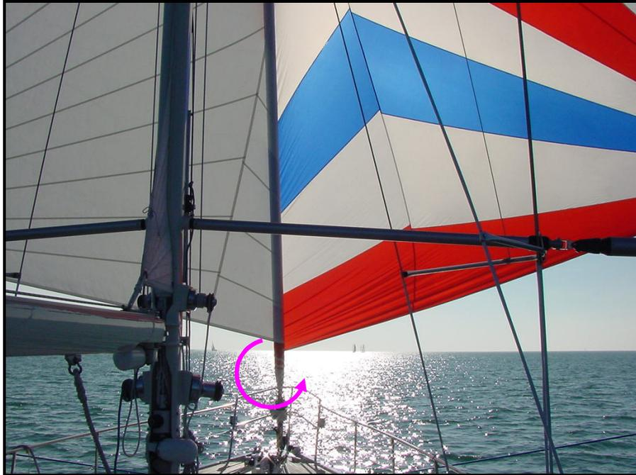
*Picture 36 – Furling the jib and the ballooner together*
