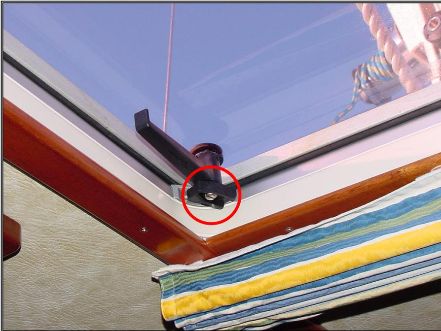
*Picture 97 – Blocking up a deck hatch*
