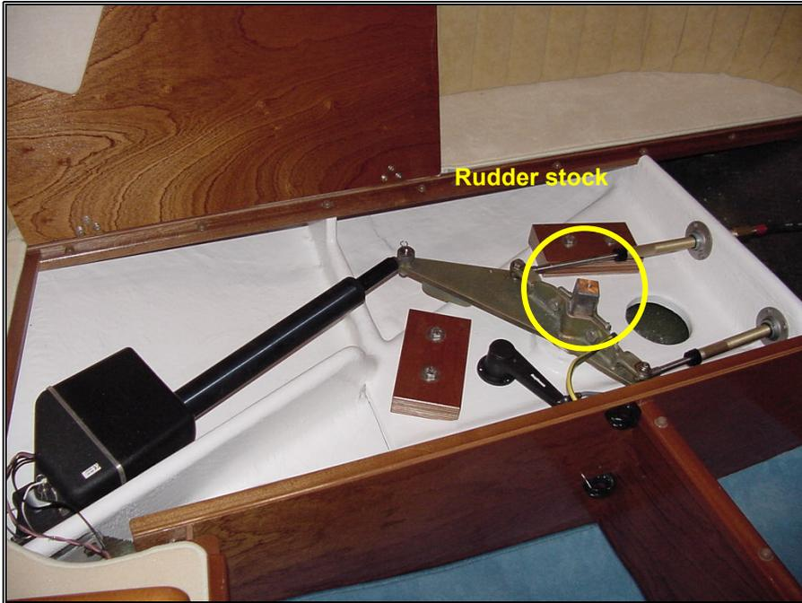
*Picture 10 – Rudder stock and automatic pilot linear driving unit*
