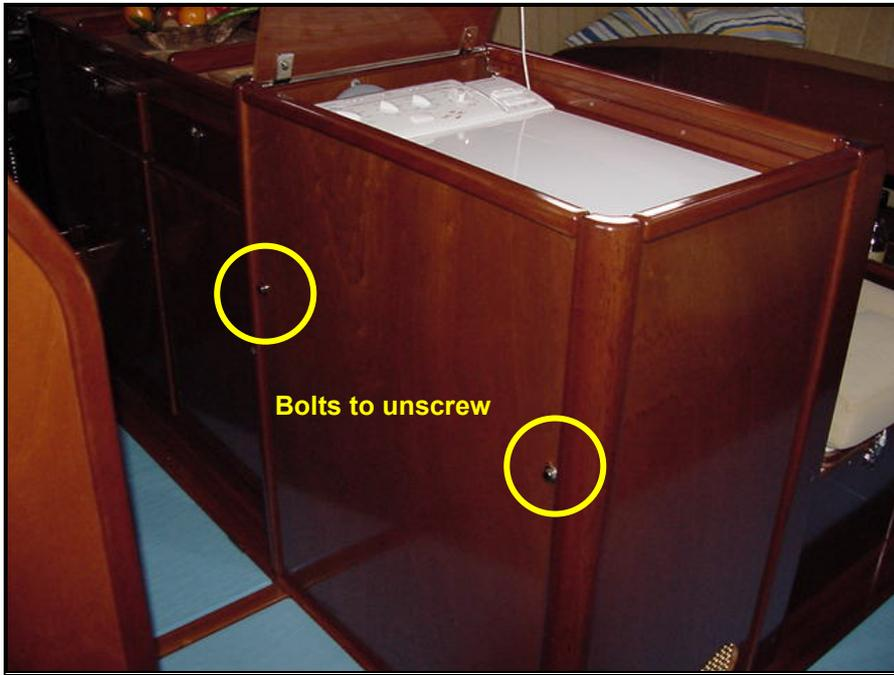
*Picture 102 – Removal of the clothes washer / dryer*
