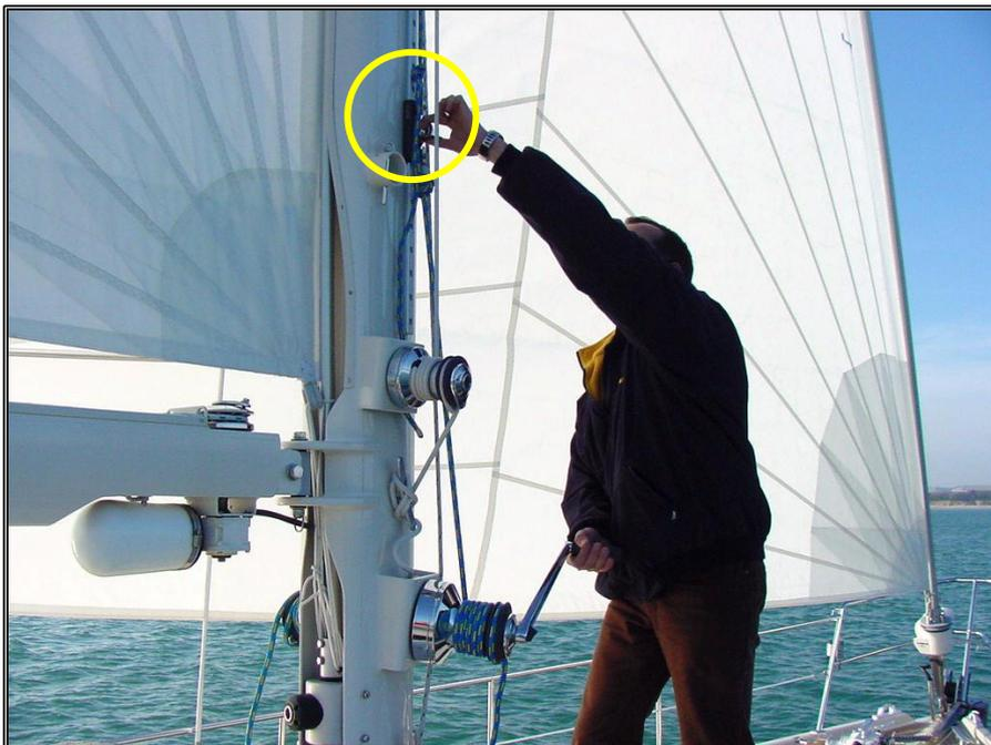
Picture 16 – Tightening the mainsail halyard
