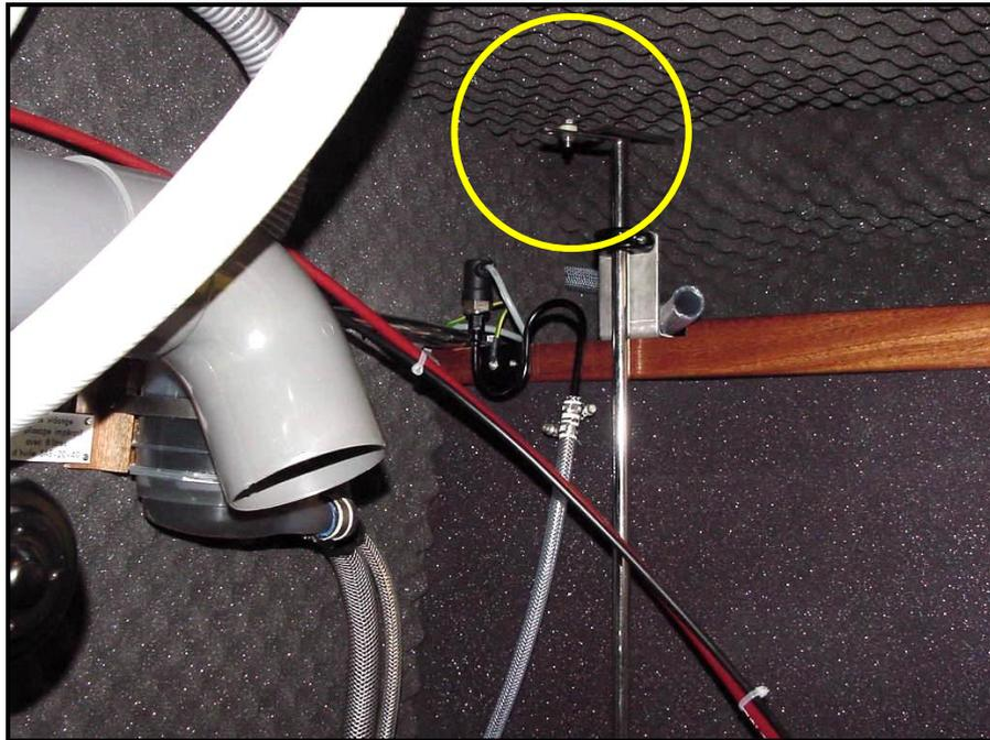
Picture 51 – Stopping gas-oil delivery from the engine room
