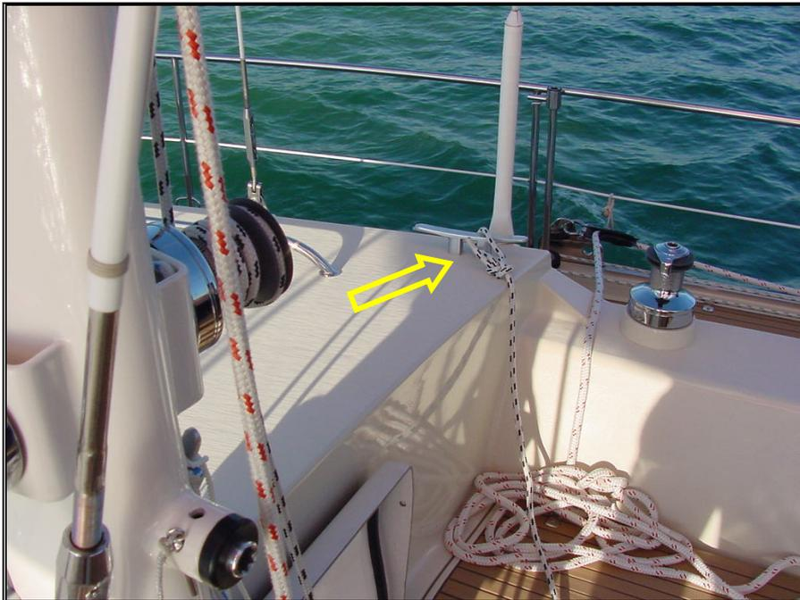
*Picture 41 – Halyard secured before hoisting*
