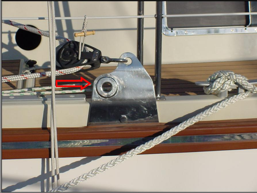
Picture 100 – Aft lift U-bolt
