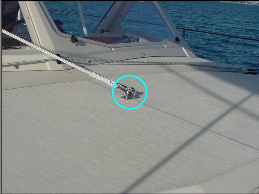
*Picture 39 – Setting the tack on the mizzen ballooner*
