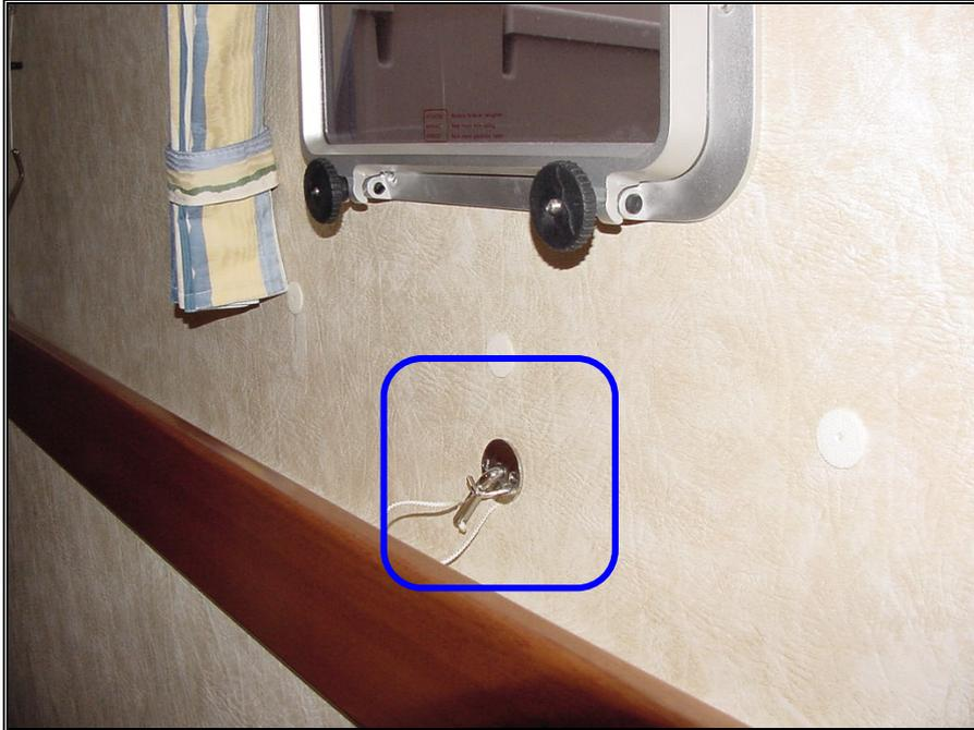
*Picture 53 – Locking the opening of the engine room's cover*
