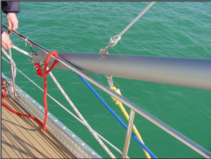
*Picture 30 – Attachment of the lines on the pole and way of jib's sheet*
