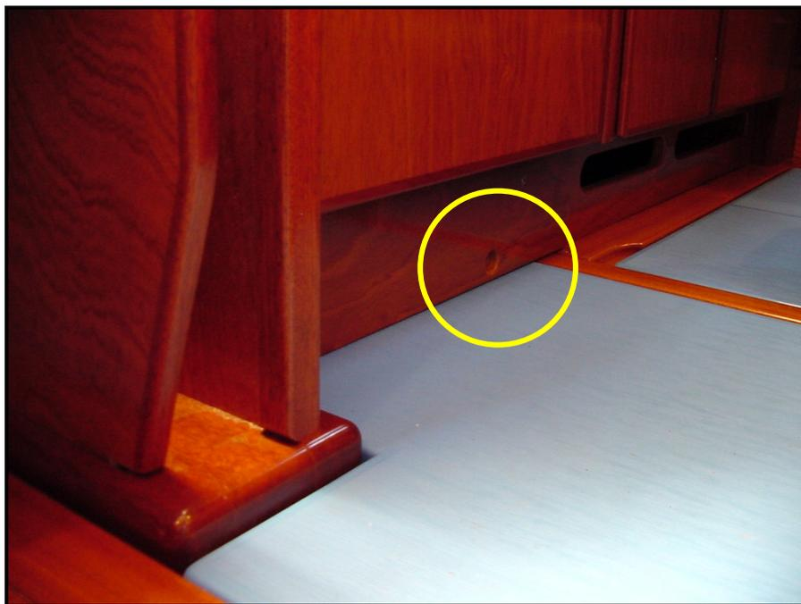
*Picture 73 – Switch for setting the speed of the fan*
