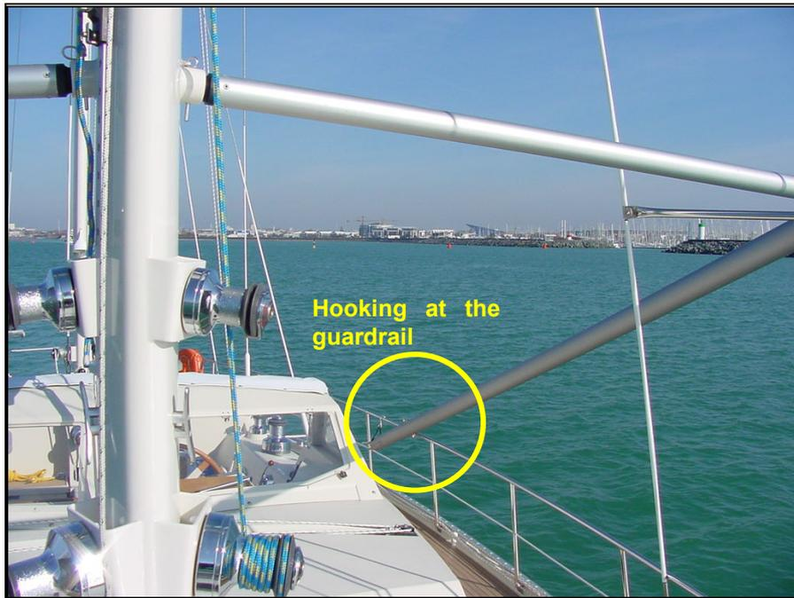
*Picture 29 – Pole hooked to the guard-rail*
